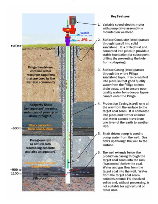
Figure 1 Basic schematic of a coal seam gas well
